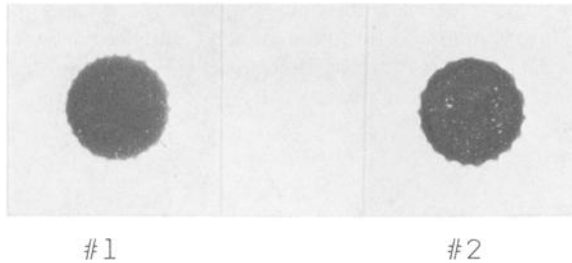
FIG. 7—The first stain, on the left, was produced by a drop of blood (approximately 26 \mu\text{L} ) falling 116 cm from a pasteur pipet. The second, on the right, resulted from a drop of blood (approximately 50 \mu\text{L} ) falling only 25 cm. The substrate was the same in each instance.
